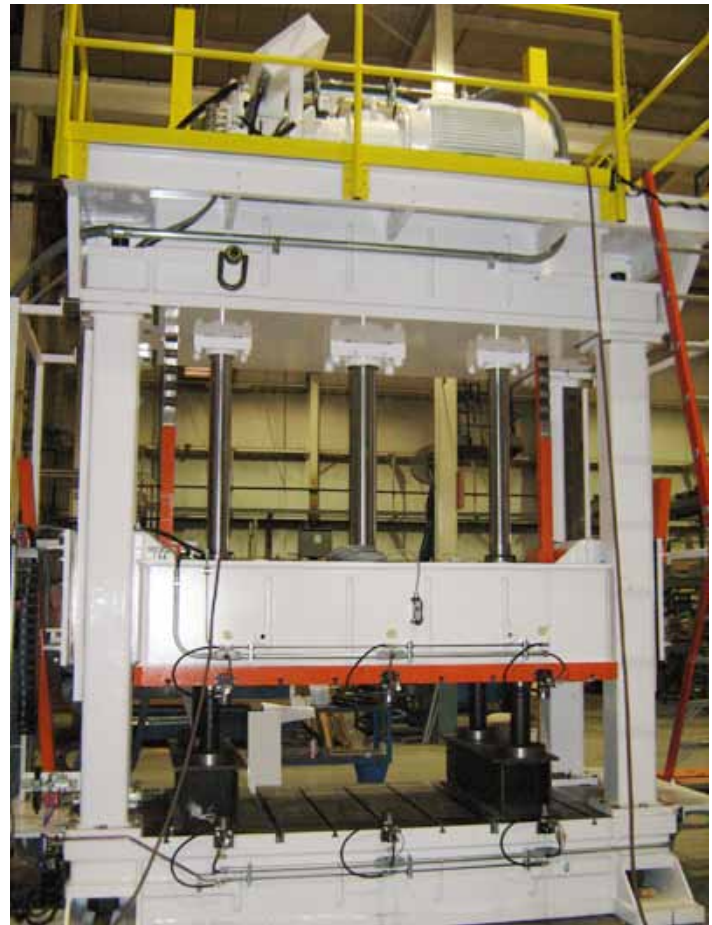
Adding load-sensing technology to Eaton piston and vane pumps and screw-in cartridge and industrial proportional valves has enabled Fabriweld presses to operate more quietly and on less electrical energy.
